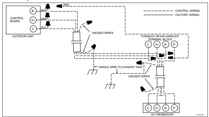
Figure 6: Typical communicating field wiring for air handler or furnace
