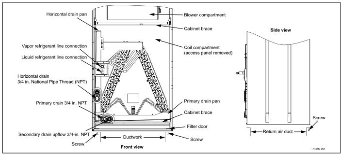
Figure 1: Return air duct attachment and component location
