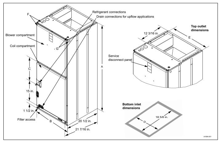
Figure 2: Return air duct attachment and component location
