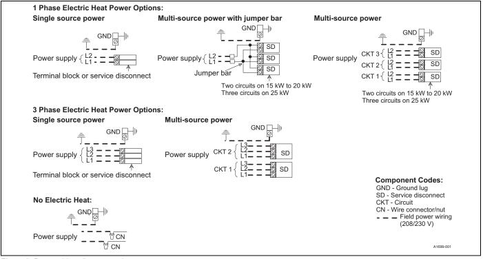
Figure 3: Power wiring - line connections
